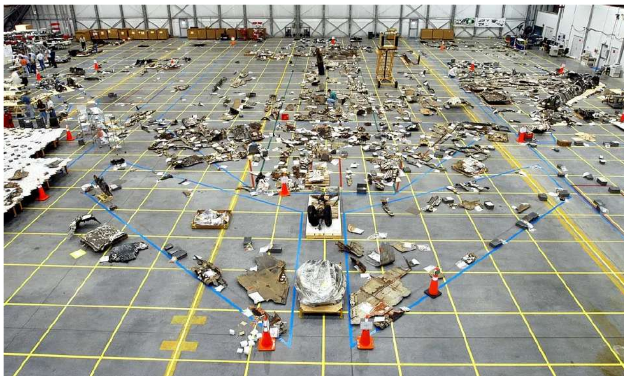
Recovered debris from the Columbia space shuttle.
